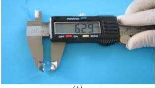
transparency of the lenses graded by using criteria adopted by Mehra and Minassian7. All the lenses were clear and transparent with no opacities. Thickness and diameter of all the lenses were recorded with digital vernier caliper. In the
