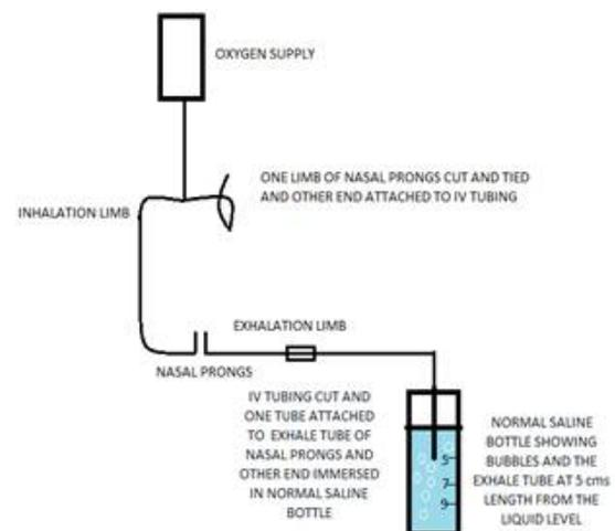
**Figure-1: Schematic diagram of indigenously prepared NB-CPAP.**
